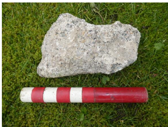
Fig. 11 A piece of lime mortar, full of inclusions, from within Lady Anne's 90-rood wall (200mm scale).
