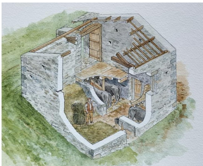
Figure 3 Cutaway image of a bank barn located in field with bank access to first floor cart entry, housing for cattle, and storage for crops (drawn by Allan T. Adams).
