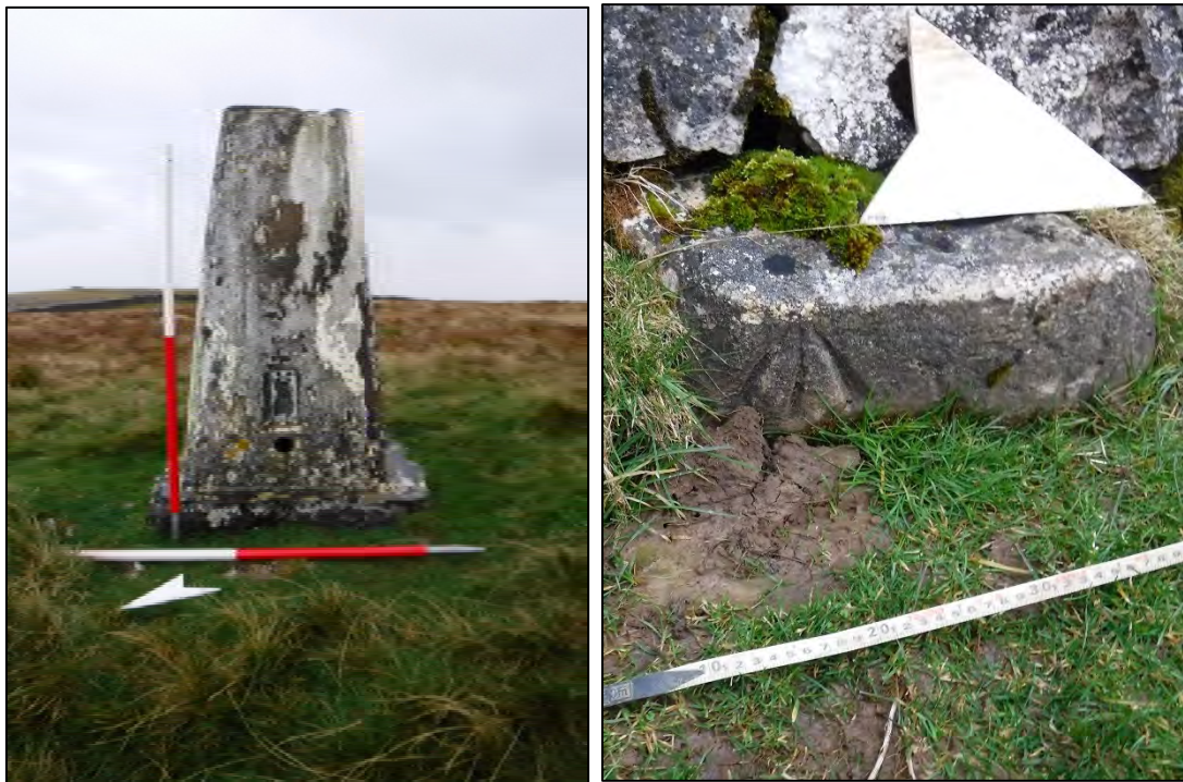
Plate 108: (left) trigonometric column D61 (looking south-east). Plate 109: (right) benchmark located at the foot of stile G326 .
