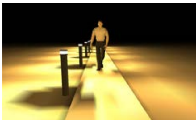
Omi-directional illumination: 10lux with 0.05 uniformity/ 25% dimming Low efficiency & High glare
