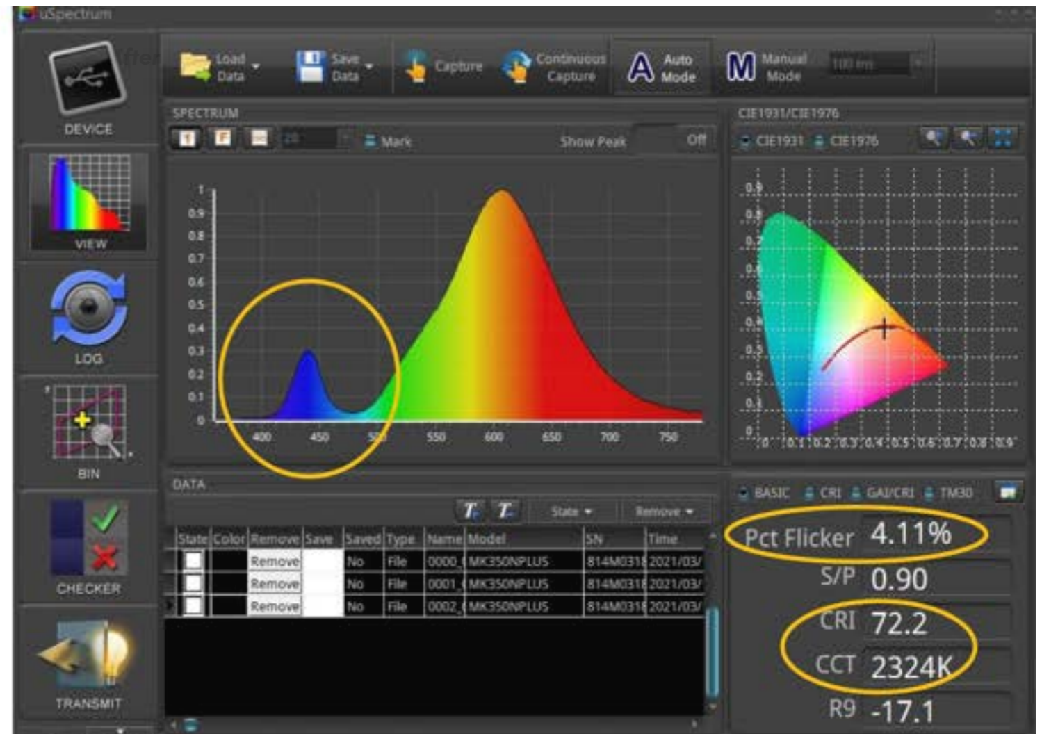
Prestegne Dark Sky Project spectral readings showing the improvement rate before & after the street lighting refurbishment. Courtesy of Brian Healy.
