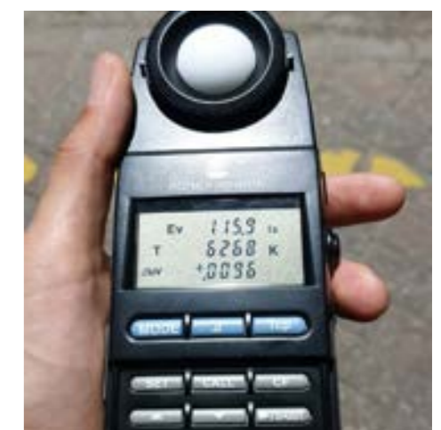
Option 4 - LUX & CCT readings *If the site is already illuminated. (See page 44 )
