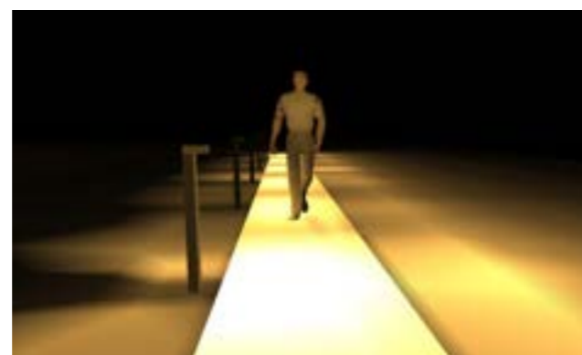
Directional illumination: 10lux with 0.2 uniformity/ 75% dimming High efficiency & Low glare
